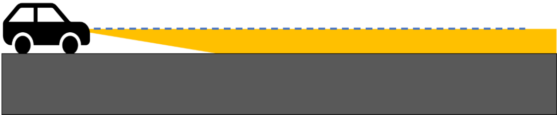
Figure 19. Proposed lower beam path of aim. With our low beam being able to vary intensity of the beam when an oncoming driver is approaching, we propose being able to aim the beam closer to the horizon such that the low beam truly has a farther reach increasing visibility.
